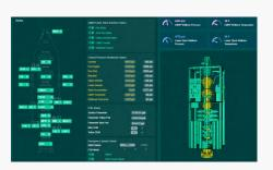
System generated event and alarm loggers which visually notify the monitoring staff to investigate and potentially initiate a failure in the Failure Propagation portion of the system
